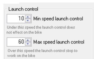
launch control switch on automatically. Until the bike does not exceed a certain speed (Max speed launch control) the strategy will keep the power under a specified value. When the bike exceed this speed, the power will be free to increase normally.
